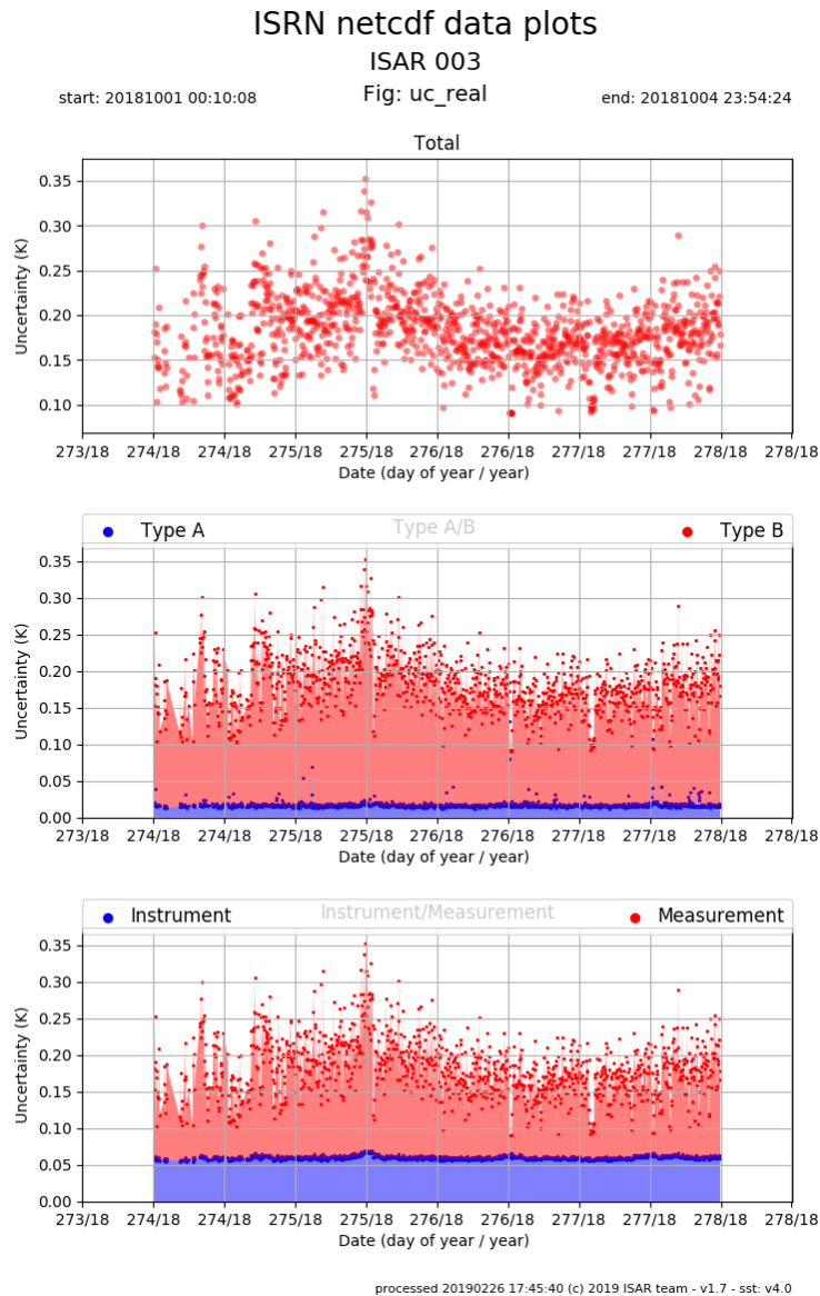
Figure 3-2: The top panel shows the total ISAR uncertainty over time, the middle panel shows the total ISAR uncertainty split into Type A (blue) and Type B (red) uncertainty, and the bottom panel shows the total ISAR uncertainty split into instrument (blue) and measurement uncertainty.
