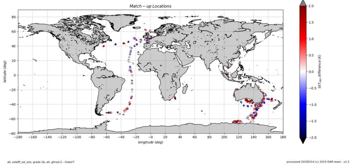
Figure 6-1 ISAR Location of the match-ups at +/- 2h and 1km coincidence for SLSTR WST dual-view SST retrievals against ISAR/SISTeR observations between August 2016 and March 2018 .
