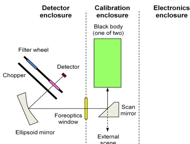
Figure 5-1: The internal configuration of the SISTeR radiometer
