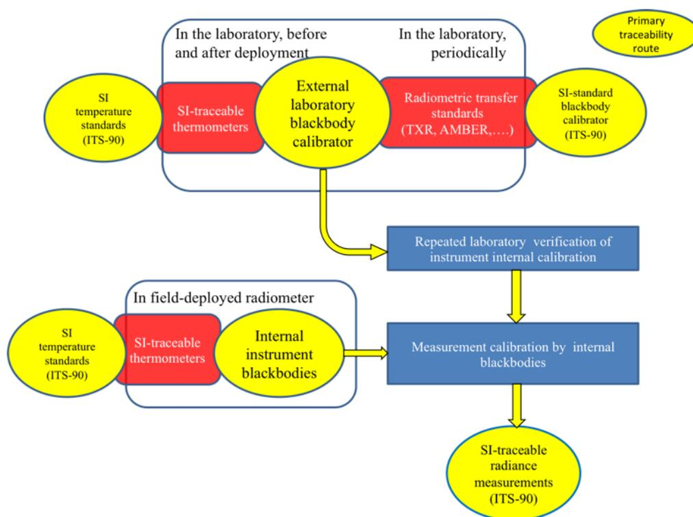
Figure 2-3 Traceability route for a shipborne radiometer (from ISSI *in situ* validation workshop).
