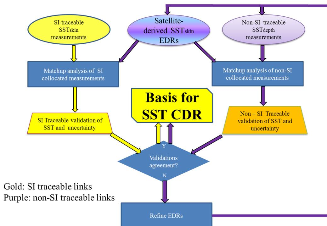
Figure 2-2 This flow diagram shows the traceability route for a SST Climate Data Record (from ISSI<sup>2</sup> *in situ* validation workshop). Shipborne radiometers cover the gold parts of the diagram.
