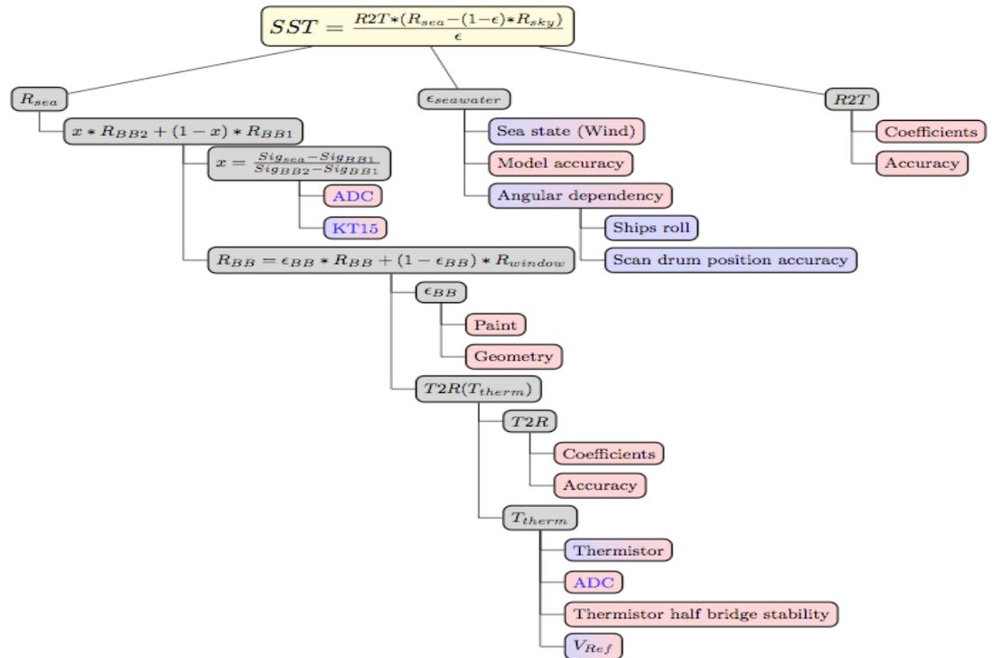
Figure 3-4: Schematic to illustrate the breakdown of the main elements of the ISAR SST processor to reveal the factors that introduce uncertainty. For clarity the  $R_{sky}$  branch has not been expanded but is essentially the same as for  $R_{sea}$ . Boxes coloured in blue represent type A uncertainties, boxes coloured in red show type B uncertainties, and boxes in red and blue contain both type A and type B uncertainties. From Wimmer and Robinson 2016.
