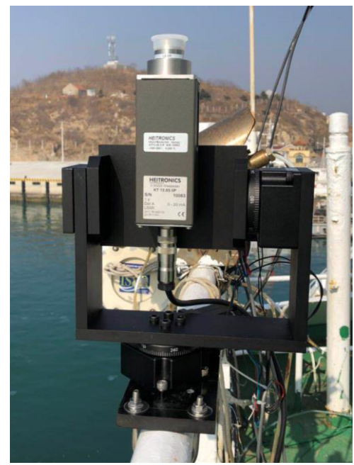
Two-dimensional rotating platform integrated with an independent infrared radiometer KT15.85
