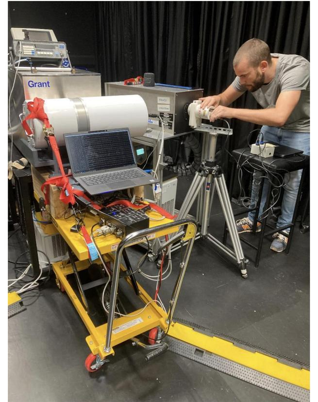
Radiometer Measurement against reference BB source at NPL during June- 2022 Radiometer Intercomparisons.
