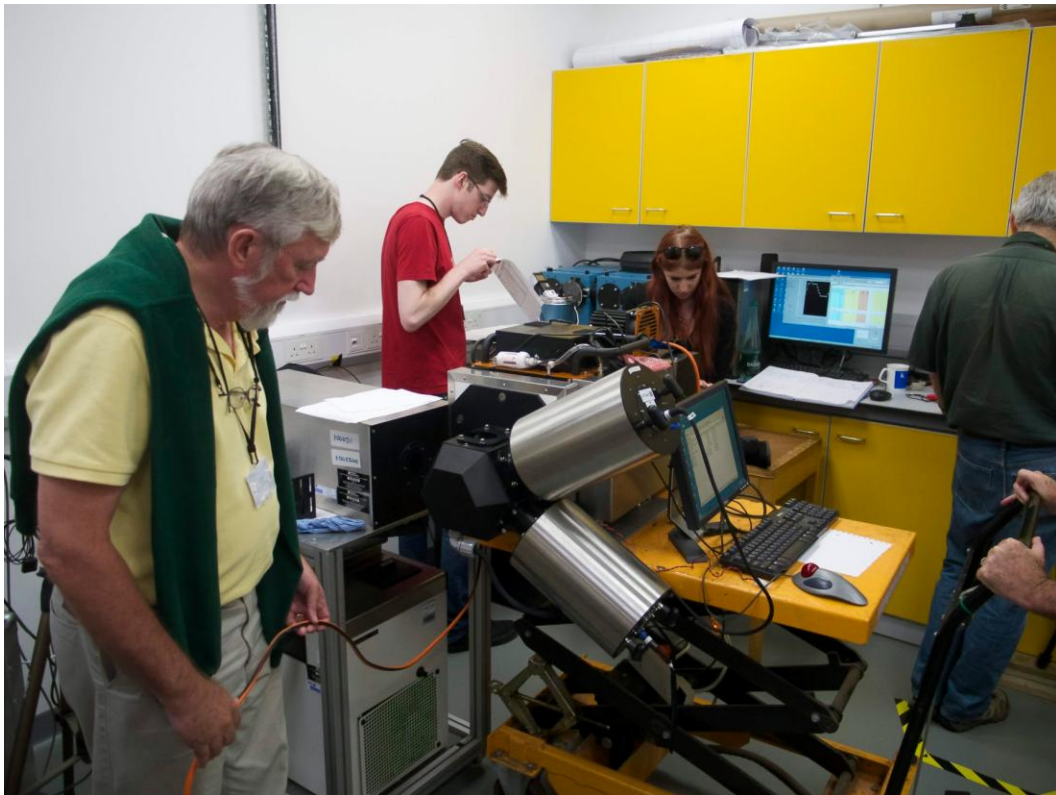
Figure 3: M-AERI mark 2 in front of the reference black body at NPL in 2016.
