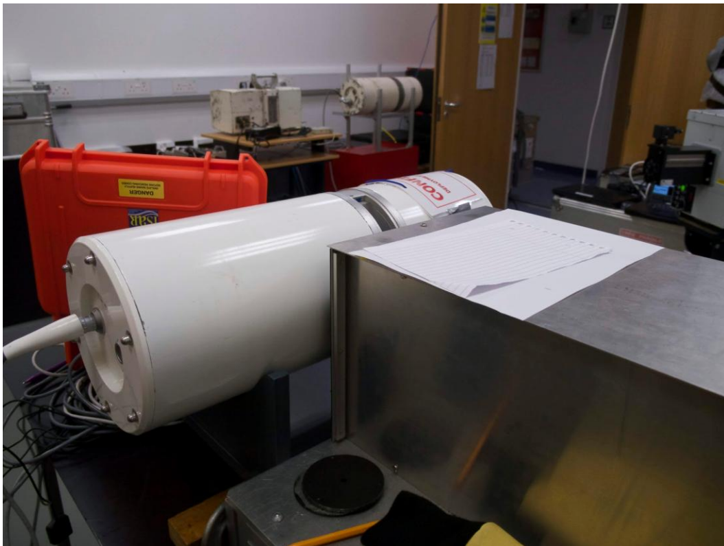
Figure 2: ISAR 03 in front of the reference blackbody at NPL in 2016.
