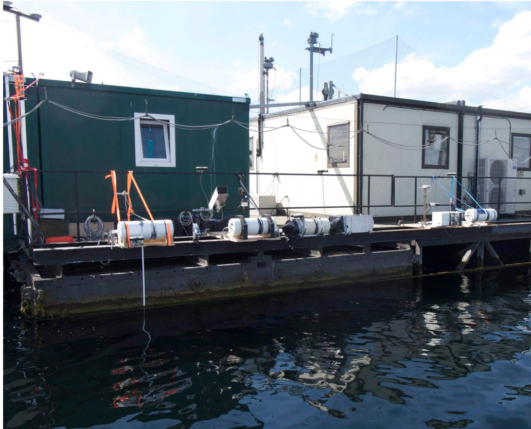
Figure 4: TIR radiometers on the NPL platform at Wraysbury in 2016.
