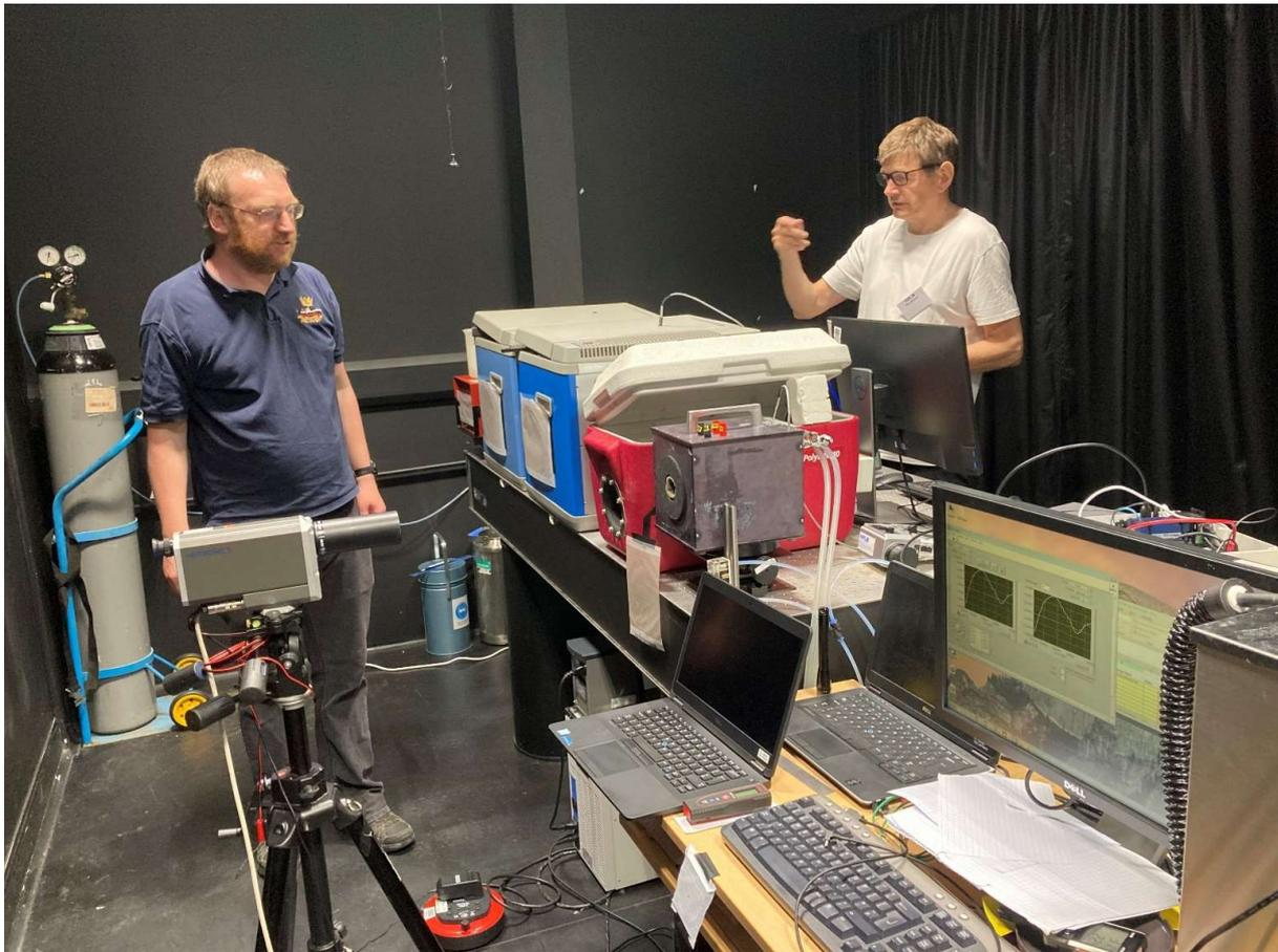
Figure 1 Radiometers measuring the reference BBs
