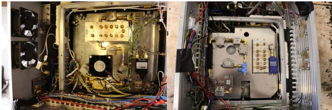
**Figure 2-8 – The refurbishment of EMIRAD-C. Left: only reusable components are left in the analogue front-end box. Right: Additional components have been fitted on a separate component layer, mounted on top of the existing component plate**
