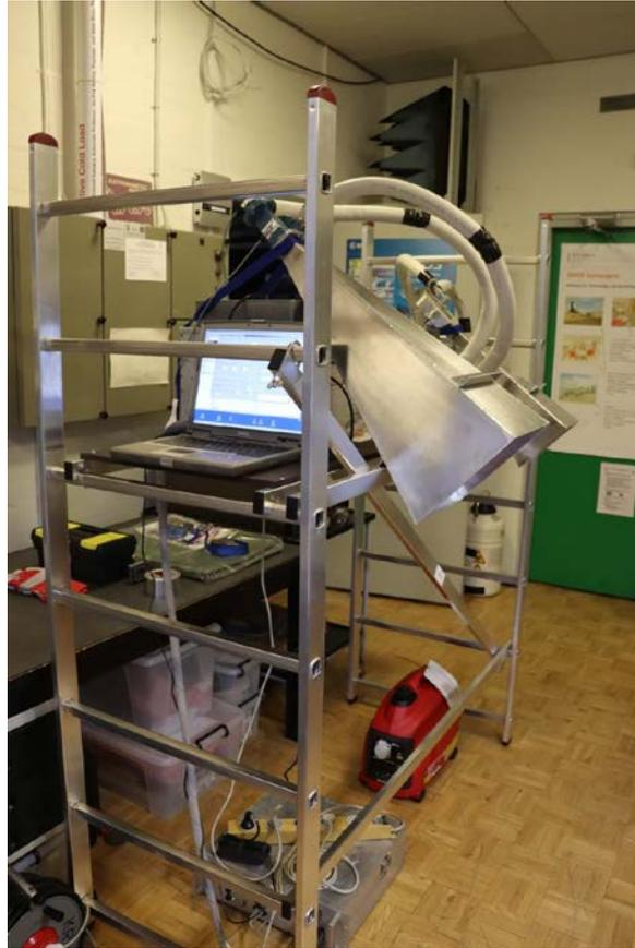
**Figure 5-2 – Scaffold with radiometers including control/storage computer and engine generator for autonomous operation at remote locations**
