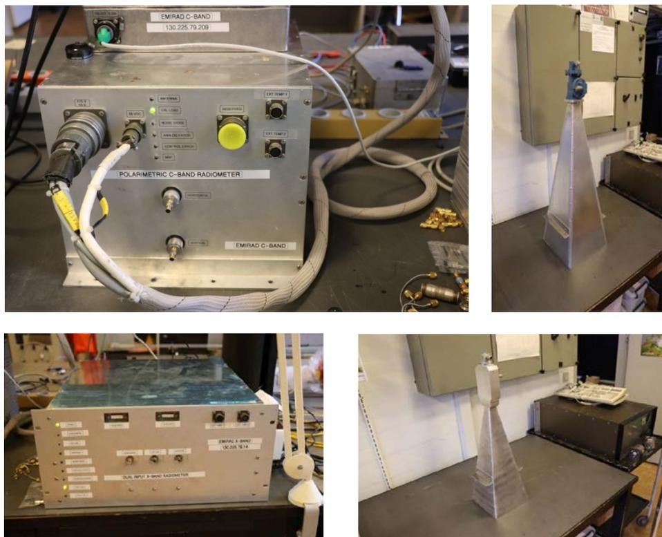
Figure 7-1 – The full hardware for measurements of brightness temperatures at C-band (upper row photographs) and X-band (lower row photographs)
