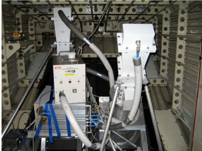
Figure 3-4 – Application of liquid Nitrogen cooled matched load in cryostat during a field campaign.
