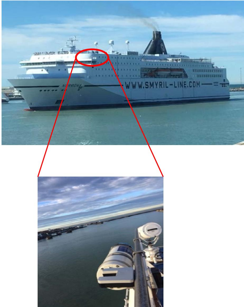
Figure 4-2: DMI-ISAR installation on board Norröna. The first deployment was made in December 2017.
