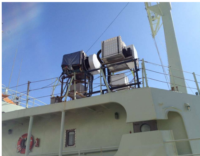
Figure 2: M-AERI mark 1 (left) and mark 2 (right) on the R/V Ron Brown.
